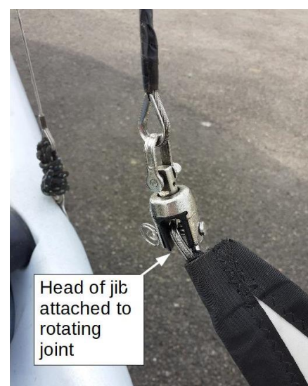
Figure 4 Rotating joint attached to head of jib
