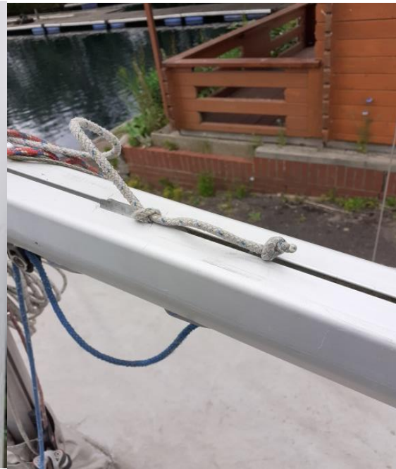
Fig11 Knot on line goes in this slot after passing through the cringle
