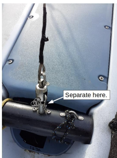
Figure 2 You should find the jib halliard stored like this
